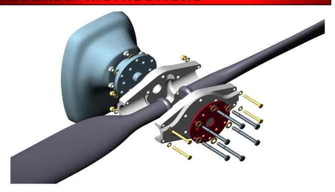
All bolts, washers and Nylock nuts used to clamp the hub plates, and attach propeller assembly to the engine should be assembled dry, without oil or moisture. Always double check you have the correct amount of threads exiting the nuts / no bottoming of threads etc. These are IMPORTANT.
