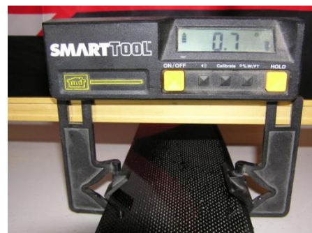
Using the Pro Angle allows the measurement to be taken through the chord line
