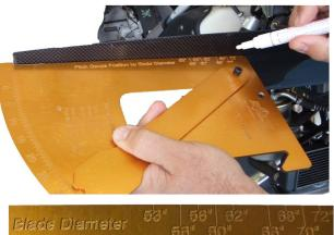
Make sure you are using the flat side of the blade. Using the Blade diameter markers on the pitch Gauge, place a mark on your blade using the marker that is the same as your blade diameter.
