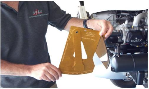
This Blade is Pitch at 17.5 degrees. The Bolly Pitch Gauge will work on most other brands of Prop as well. Use the torque setting on the pitch Gauge to re torque the bolt, if using a Bolly Prop.
