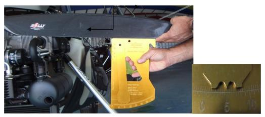
Move the blade up or down until the Pitch Gauge reads 0 degrees as per fig below. Now your blade is level.
