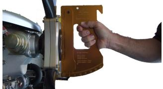
1 Place straight edge of Pitch Gauge against the prop Hub. As shown. Once the Pitch Gauge reads 0 degrees the Hub is level. You may need to place blocks or similar under the nose or tail wheel until the Gauge reads 0 degrees. This will ensure that the Pitch reading taken from the blades is accurate.
